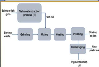
Figure 1: Astaxanthin extraction process using fish oil
