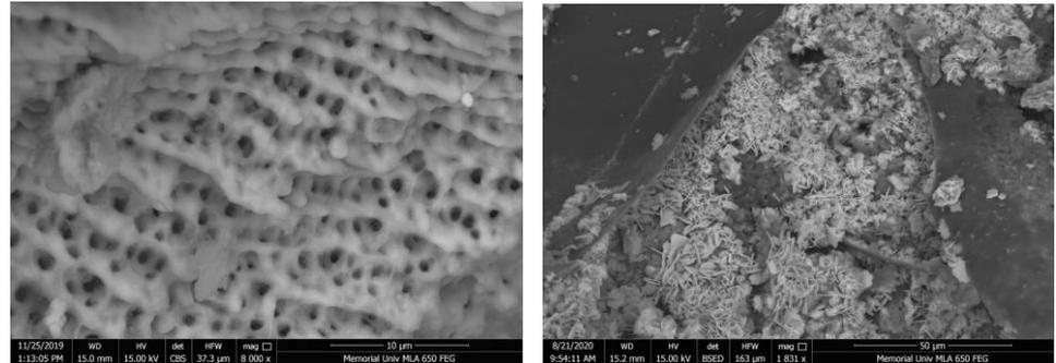
Left: Biochar pre-adsorption, Right: Biochar post Adsorption
